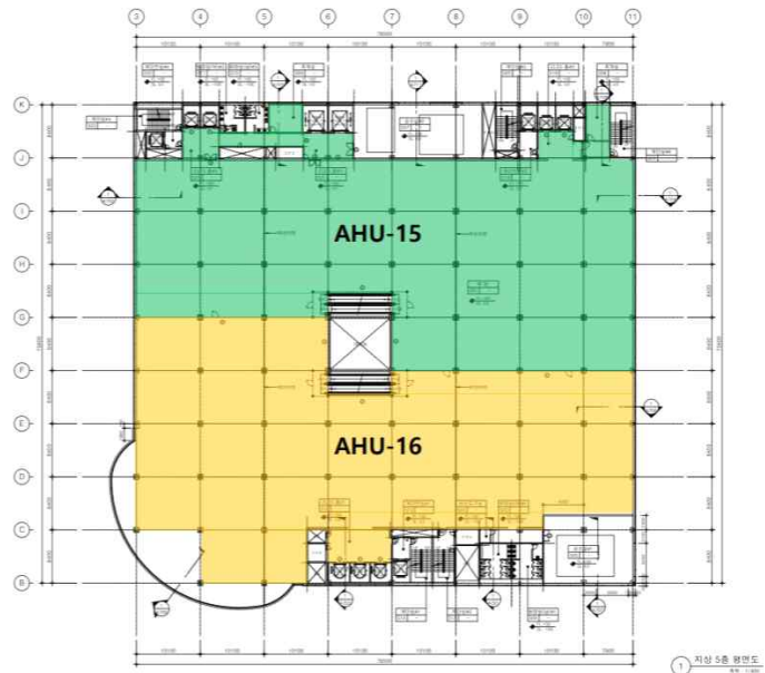
Fig. 8 Air conditioning zones for AHU-15 and AHU-16
