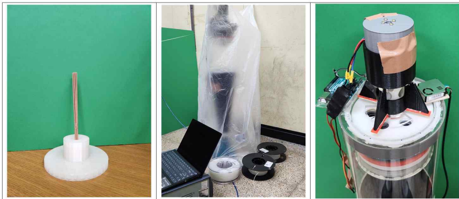
Fig. 6 Particulate matter generation through incense burning (left); air purification validation test set-up (middle); PM sensor installed at the outlet (right)
