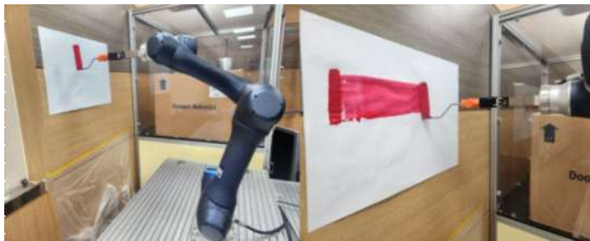
Fig. 6 Robot's paint contacting in experiment
