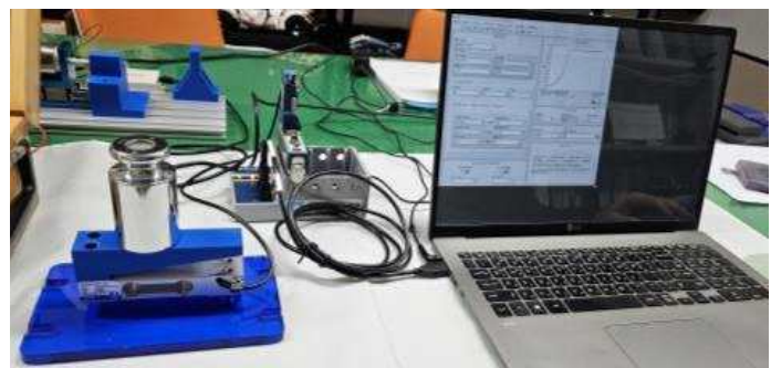
Fig. 5 Calibration of load cell with balance weight
