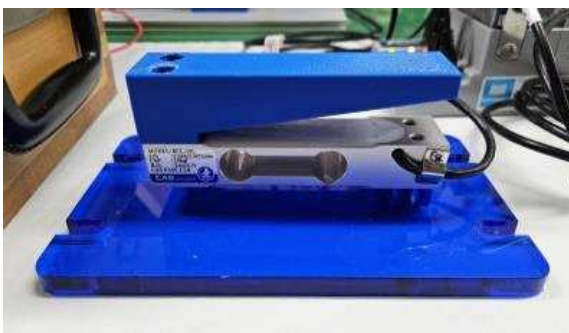
Fig. 4 Load cell with Jig
